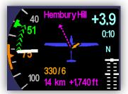
This shows the block speed (based on MC and the polar), the classic speed-to-fly (based on MC, polar and the current airmass). Speed direction (speed up/ slow down) is done with coloured chevrons and the user should be able to correlate the vario audio / STF tones (or quiet) with what they are seeing on the screen.
